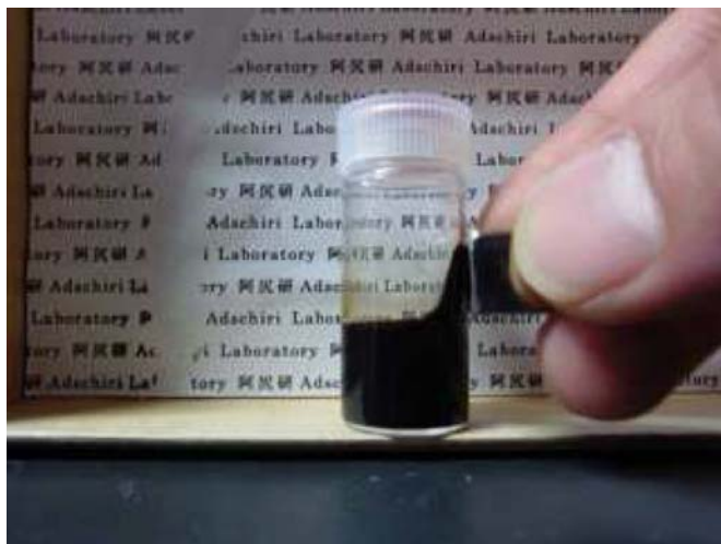
FIGURE 53.6 The magnetic response of raspberry-like magnetite nanoparticle assembled clusters.
