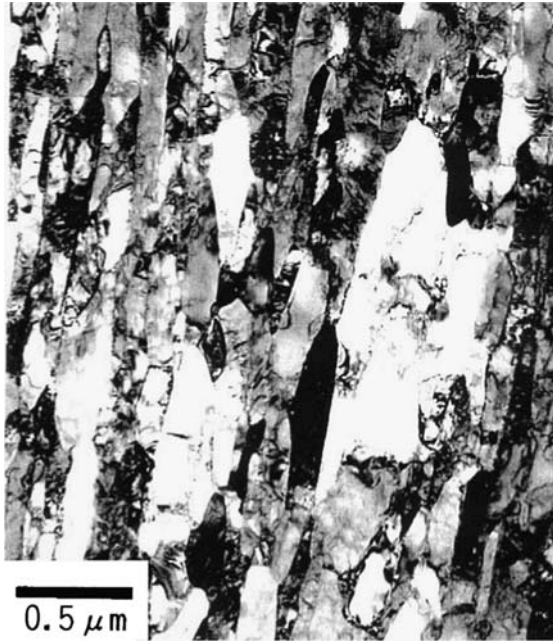
FIGURE 4.4.19 TEM micrograph of ultralow-carbon steel after 10 passes of side extrusion.
