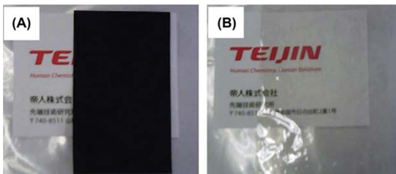
FIGURE 65.3 Appearance of (A) poly(m-phenyleneisophthalamide) (PMPIA)/multiwall CNT (99/1 w/w) and (B) PMPIA/boron nitride nanotube (99/1 w/w) cast film.
