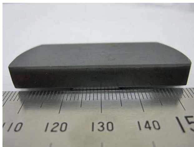
FIGURE 68.7 A joined couple of monolithic AlN and AlN/ceramic-bonded carbon.
