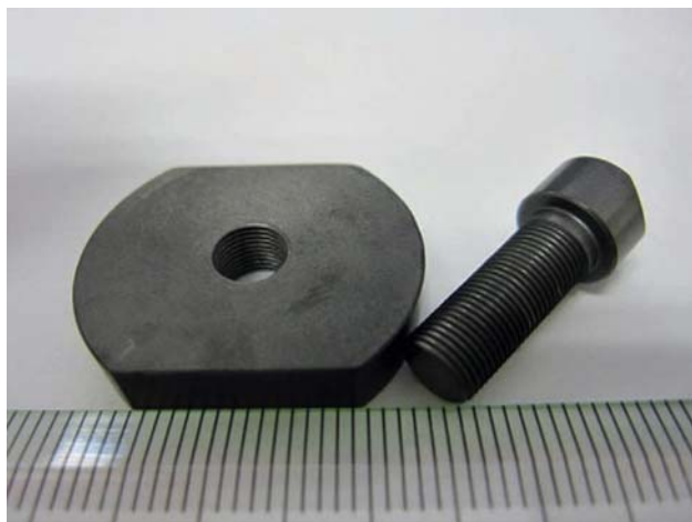
FIGURE 68.6 A fine nut and bolt made of SiC/ceramic-bonded carbon.
