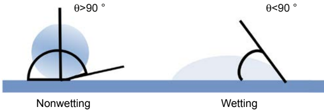
Figure 2.1 Water contact angle for hydrophobic (nonwetting) and hydrophilic (wetting) surfaces.
