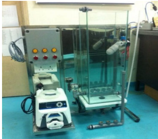
Fig. 2. Ultrafiltration Membrane System.
