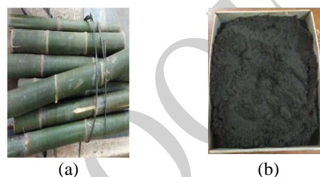
Figure 1. (a) Raw material, (b) activated carbon of betung bamboo
