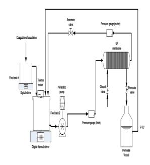
Figure 1 An example figure of the application of hybrid membrane system
