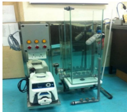
Fig. 2. Ultrafiltration Membrane System.
