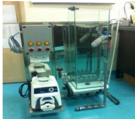
Fig. 2. Ultrafiltration Membrane System.
