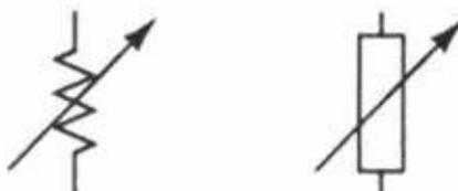
Gambar 2.5 Simbol Resistor Trimpot (Ahmad, Elektronika Dasar, 2007)
