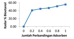
Figure 2: Comparison of the number of adsorbent ratios used with bioethanol produced at 250°C.
