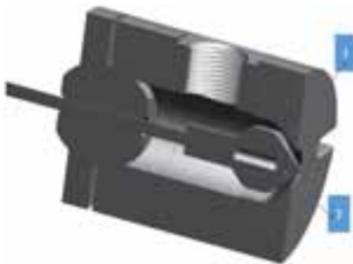
Fig. 4. Adjustable nozzle for experimental ejector: 1—Nozzle; 2—Regulating needle.
