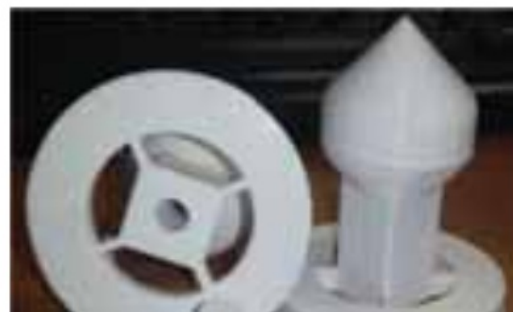
Fig. 6. Regulating needle printed on a 3D-printer.
