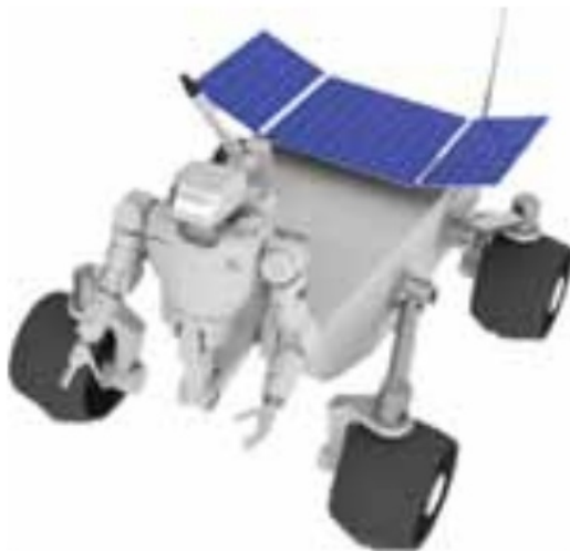
Fig. 11. Lunokhod with the torso part of an anthropomorphic robot for research of stony, rocky rocks and with the possibility of repair (of itself and other lunar technology).
