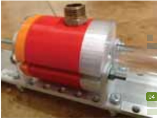
Fig. 7. The printed adjustable nozzle.
