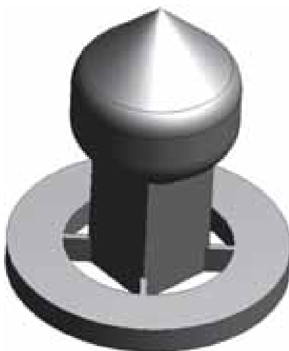
Fig. 5. 3D model of the regulating needle.
