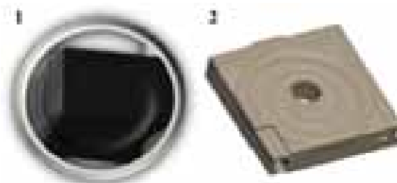
Fig. 3. Sealed container for delivery of samples to Earth (1). Cassette for storing a stratified regolith column (2).
